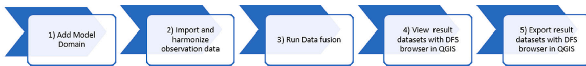
Fig. 4. Typical work-flow in the DFS system.
